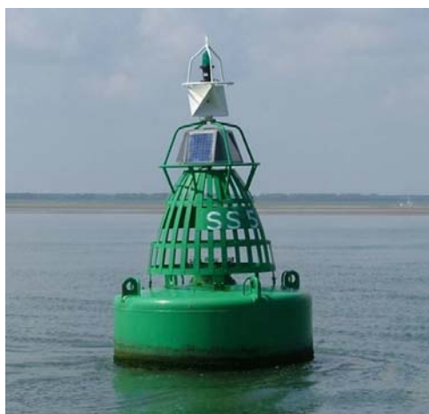
Figure 8 Lattice construction of a lateral buoy
